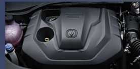
1.4L Turbocharged Gasoline Direct Injection (TGDi) engine Max. power: 160 ps / 5,500 RPM Max. torque: 260 Nm / 1,500-4,000 RPM
